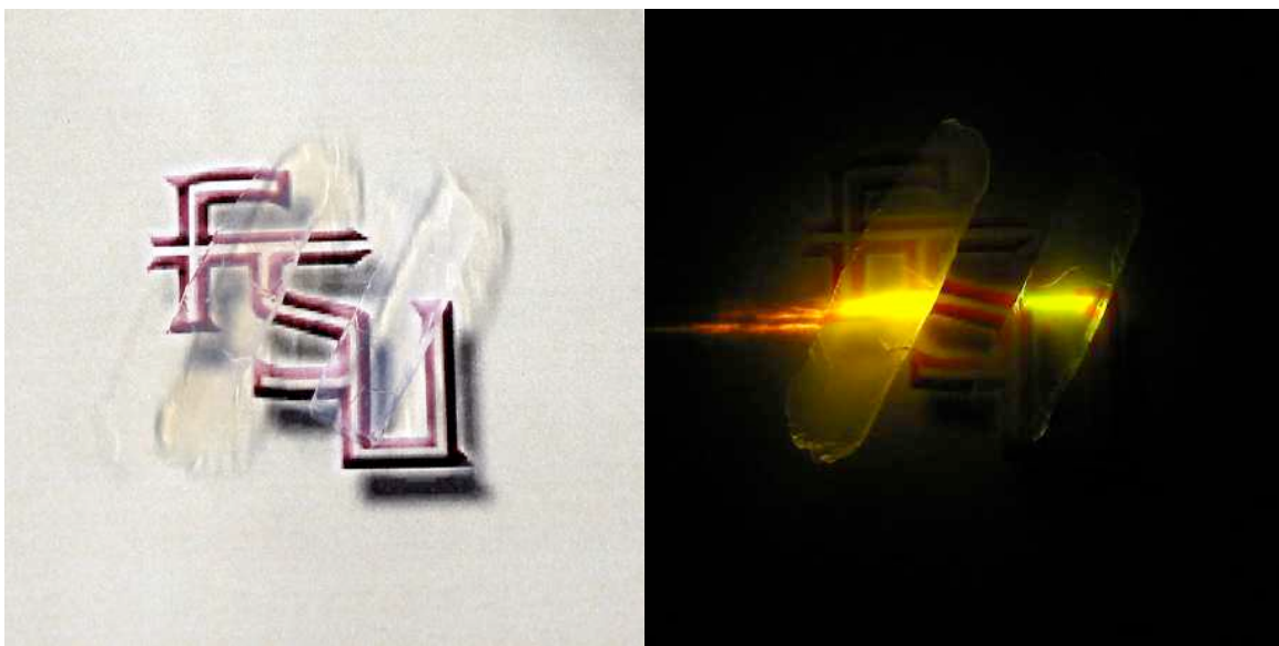
Figure 3.3 – 6 nm and 2.5 nm aerogels seen in room light and under 488 nm laser excitation as seen through a 488 nm filter. Luminescence seen in photo is from quantum dot emission.
