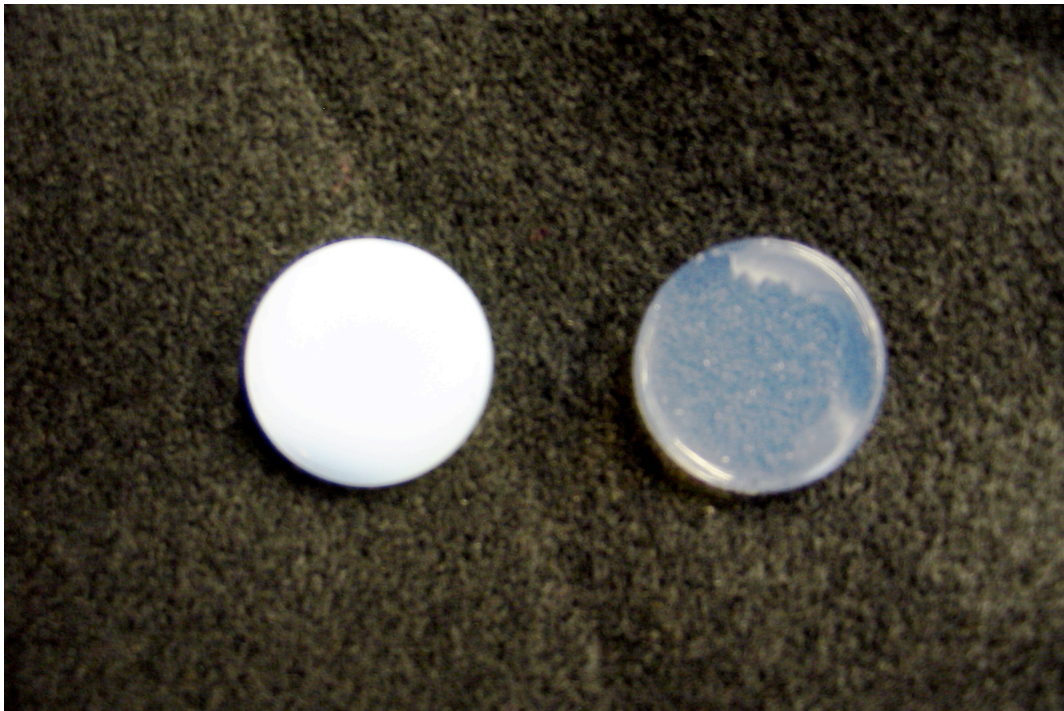
Figure 2.5 - Two CdSe/ZnS Xerogel monoliths prepared with identical quantum dot concentration and conditions. Gel on left has gone spontaneously cloudy while gel on right is clear.
