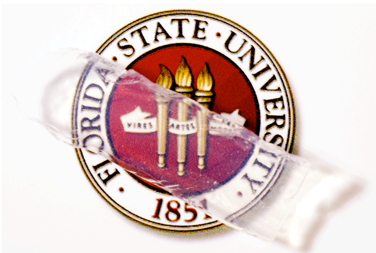
Figure 3.1 - Silica aerogel containing 2.5 nm CdSe/ZnS quantum dots.
